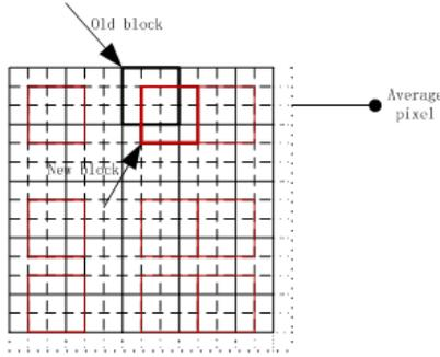
Figure 4. The shift block in method 1
