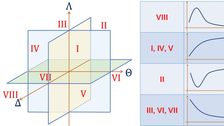
**Figure 2.** The planes  $\Delta = 0$ ,  $\Theta = 0$ , and  $\Lambda = 0$  divide the space into eight octants. The monotonicity of  $m(t)$  is determined by the octant that the point  $(\Delta, \Theta, \Lambda)$  lies in.
