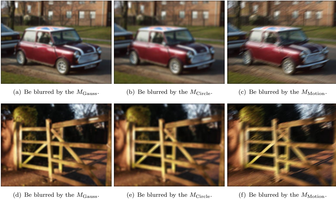
Figure 3. Images that have been blurred by the matrices M_{\text{Gauss}} , M_{\text{Circle}} , and M_{\text{Motion}} respectively.
