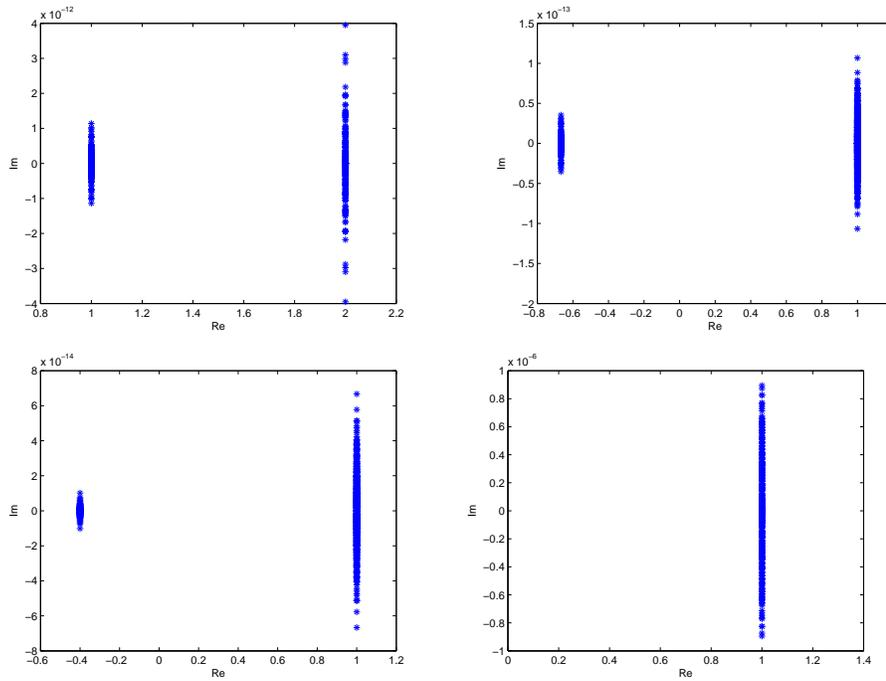
**Figure 4.** The eigenvalue distribution for the block triangular preconditioned matrix  $\mathcal{P}_t^{-1}\mathcal{A}$  when  $t = -0.5$ (the first),  $t = 1.5$ (the second),  $t = 2.5$ (the third) and  $t = -1$ (the fourth, the optimal parameters), respectively. Here,  $h = \frac{\sqrt{2}}{18}$ .
